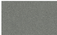
Weathered Galvalume SR=.44 E=.63
